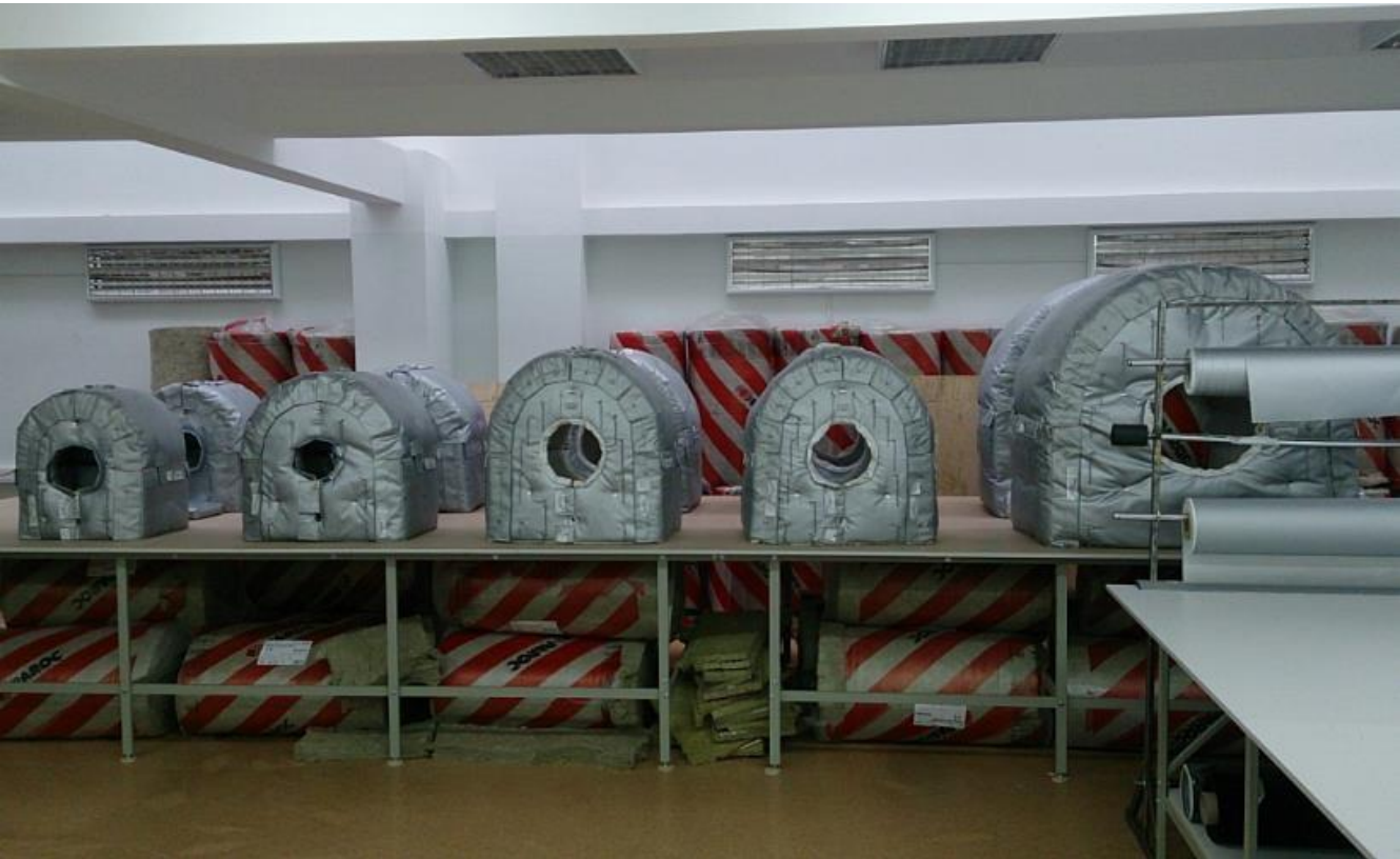
23. Oil producing company. Thermal insulation of high temperature pumps.
